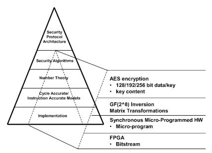
Figure 3. AES processor within the security pyramid.
