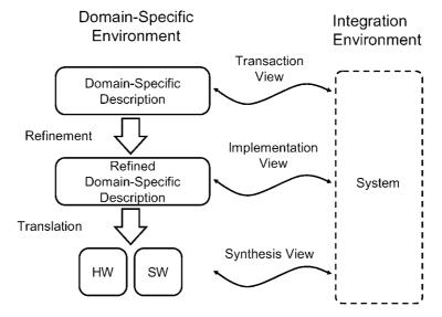
Figure 5. Domain specific design flow.
