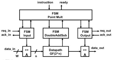
Figure 4. Elliptic curve encryption processor.
