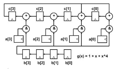
*Figure 7.*  $GF(2^4)$  bitserial multiplier.
