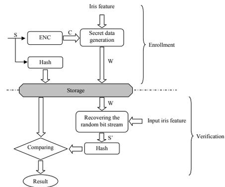
**Fig. 2. Template-protected iris matching algorithm**
